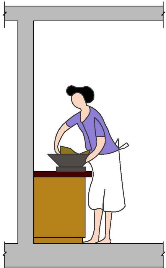
Correct Design of Cabinet Bases for Convenient Cleaning and Working (>8cm)
