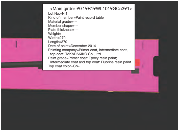
Fig. 6 Maintenance Information (Paint Record Table)
