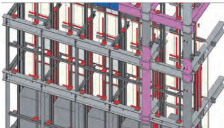
Photo 3 BIM-based consensus of steel-frame members for elevator equipment (red) and steel-frame model (grey)
